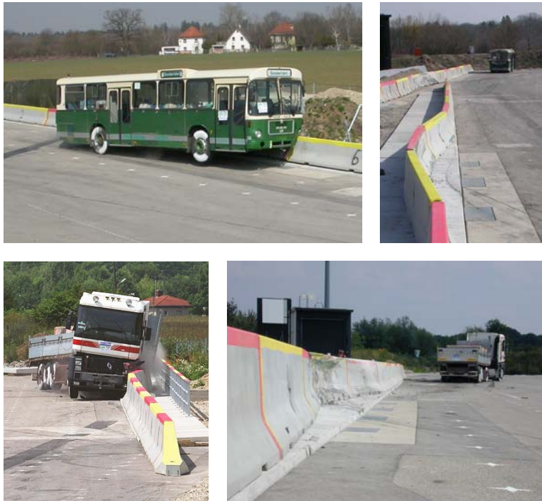
Figure 2: H2/TB51 test with 13 ton bus and H4b/TB81 test with 38 ton truck
